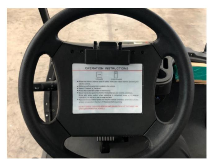
• **Step One:** Remove the front plastic cover of the steering wheel. Pull the top of the plastic cover towards you, you will hear the clips release. The cover can be set aside at this time.
