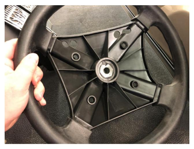
To re-install, place the steering wheel on the splines of the shaft. Tighten nut by hand and then tighten with ratchet/Impact driver. Place center cover over steering wheel and press firmly at the bottom and top.
