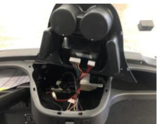
At this point you will now have access to the back of each headlight. You will need to reach in as far as you can to reach the knobs. It is a very tight fit and the knobs are snug. If you cannot get the knobs to turn you can try and use a very small set of channel locks to get a better grip on the knob to turn.
