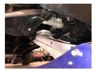
The center frame directly behind the steering rack.
