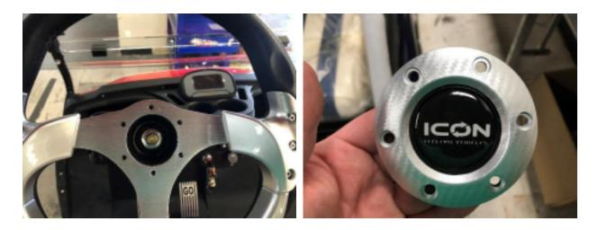
Pictured is the steering wheel with the trim ring and center cap removed
