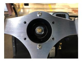
• **Step Three:** Using your extension, 18mm socket, and ratchet, remove the steering shaft nut. Thread the nut back on about 3 threads and give the steering wheel a few firm pulls. This should free the steering hub from the shaft and the assembly can be removed.
