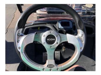
• **Step One:** Remove the 6 Allen head screws around the trim ring. The trim ring, the center button, and the steering wheel will all be free from the steering hub.
