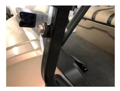
• **Step Three:** With all of the hardware removed, the windshield can be removed by pulling the windshield towards you and prying open the black plastic retainers on the roof support bar.
