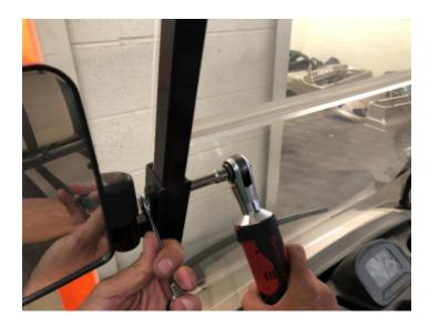
• **Step Two:** Remove the nuts and bolts that the windshield rests on.
