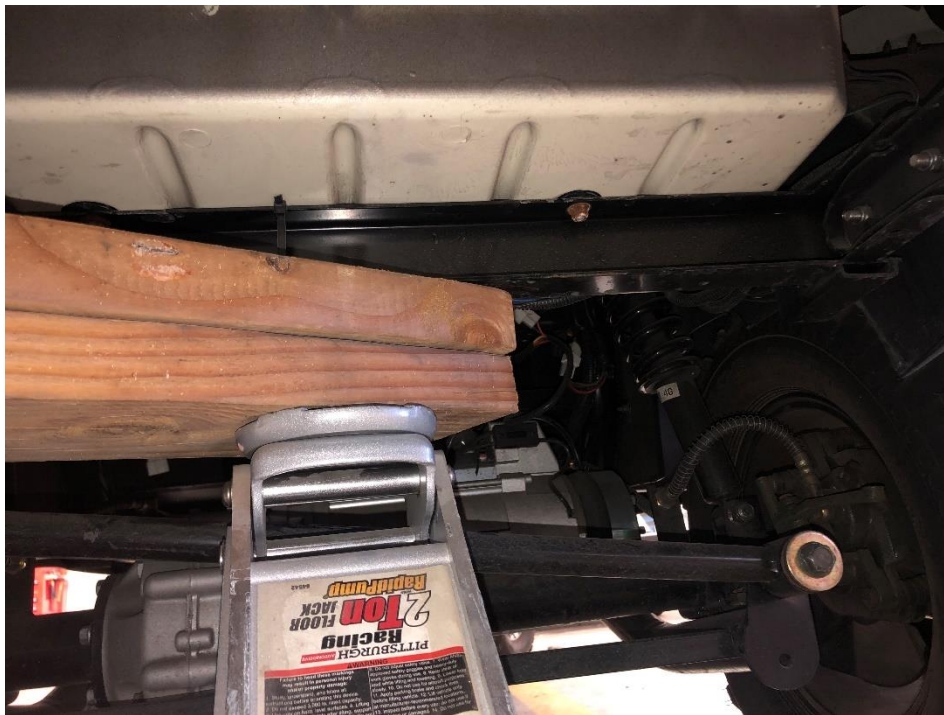
*REAR OF CART-CROSS BRACE OF FRAME JUST BEHIND THE REAR BUMPER*
